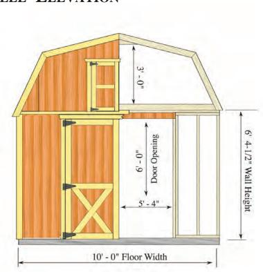
**Roof System:** 2x4 trusses spaced 24" on center, (see engineered truss drawing for load ratings). 7/16" OSB roof sheathing. *Shingles by owner*.
