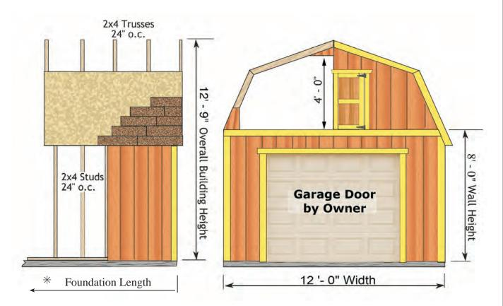
**Wall Framing:** Constructed from 2x4 pre-cut wall studs spaced 24" o.c. Bottom plate, top and tie plate. Door Header is a 2x10.
