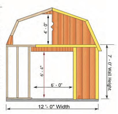
**Roof System:** 2x4 trusses spaced 24" on center, (see engineered truss drawing for load ratings). 7/16" OSB roof sheathing. *Shingles by owner*.
