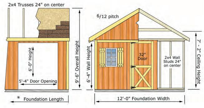
\*\* Foundation length is the same as building length. Example; 16' building length = 16'=0" foundation.
